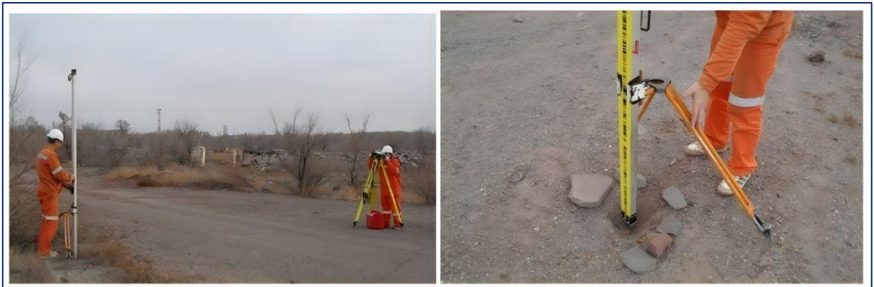
Figure 2 –Measuring the subsidence of the earth's surface using a benchmark
