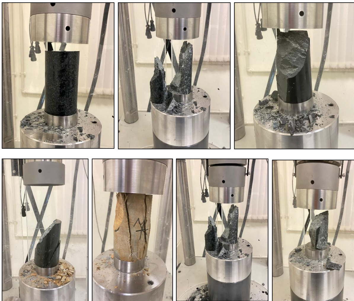
Figure 1 – Destroyed rock samples
