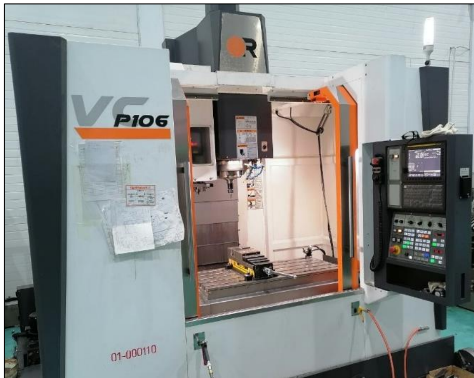
Figure 1 – Vertical machining center (V-Center P76) with CNC
