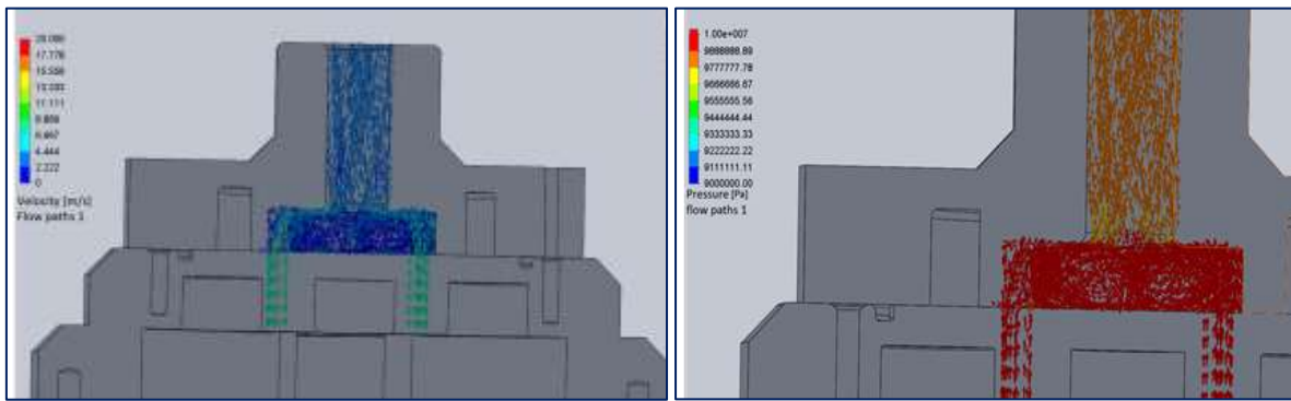
Figure 4 - Fluid velocity (a) and pressure (b) distribution at the transition radius of 15 mm in the manifold
