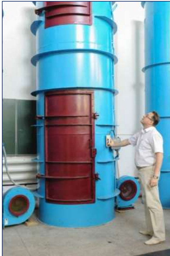
Figure 1 - Experimental-industrial sample of cargo pneumolift for buildings and constructions
