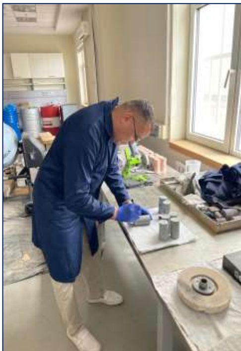
Figure 1 – Preparation of cores to determine the strength of rocks for uniaxial compression
