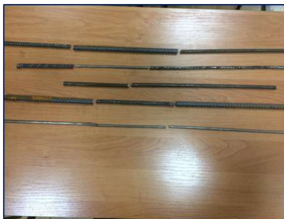
Figure 3 – Preparation of workpieces for welding
