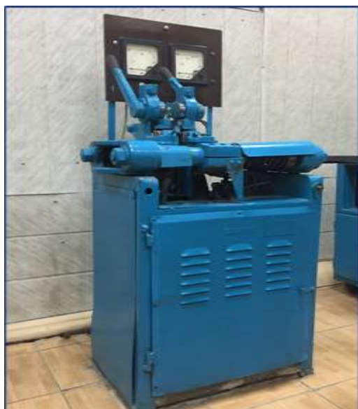
Figure 1 – The process of butt contact welding on the machine “MSR-25”
