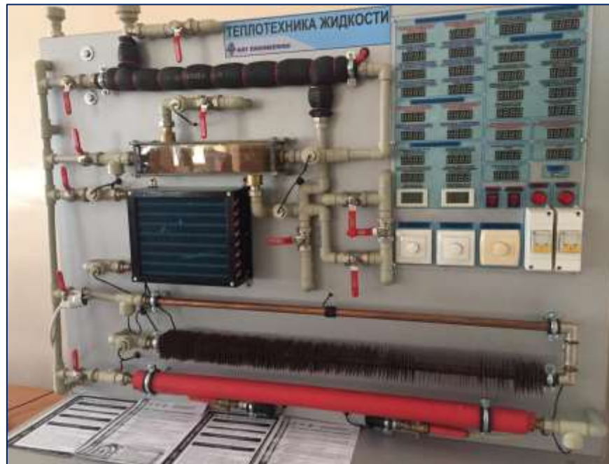
Figure 1 – Test laboratory bench for studying liquid thermal state that consists of a pipeline with thermal insulation
