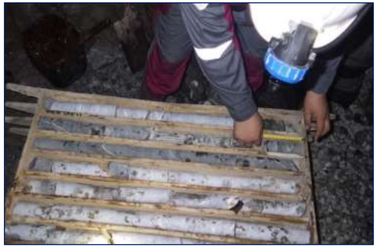
Figure 2 - Measurement of cores for RQD determination at Zholymbet field
